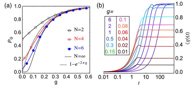
FIG. 2. (a) The probabilities to remain in the ground state at different  $g$  and  $N$ . Solid curves and the limit  $N \rightarrow \infty$  (black dashed curve) are predictions of Eq. (12) and point markers are the numerical results [19]. (b) Time dependence of computation accuracy. Solid curves are results of the numerical solution for the Hamiltonian  $\hat{H}_{\text{BCS}}(t)$  with  $N = 12$ ,  $S_{\text{tot}}^z = 0$ , and the same  $\varepsilon_j$  as in Fig. 1(b).
